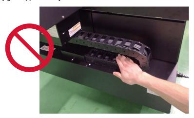
Keep away from the area that the gantry moves while printer is in operation.
